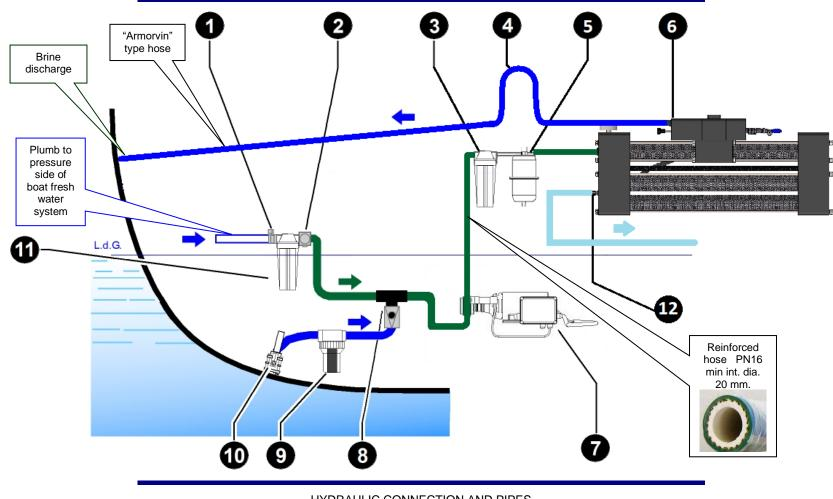
HYDRAULIC CONNECTION AND PIPES FIG. 4-7
