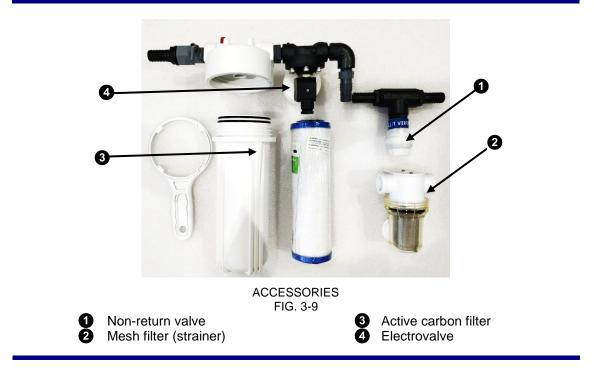
Active carbon filter. This filter is connected between the fresh water pressurized system of the boat and the electro valve on the filter holder. A manual valve positioned on the filter inlet allows replacement of the cartridge without depressurizing the fresh water system of the vessel.
