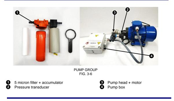
**Pressure transducer.** It is hydraulically connected to the pump group. It stops the system if the pump pressure exceeds 14 bar or if it doesn't reach 1,3 bar.
