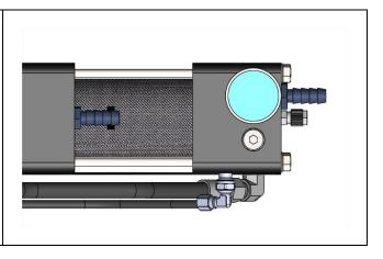
If the average pressure exceeds the above range, it is necessary to check the membranes cleanliness. If the pressure exceeds the abovementioned range, it's highly likely that the membranes are dirty or clogged, and it is necessary to perform a cleaning with the chemical SC1. If the cleaning with SC1 is not enough to reduce the pressure, it might be necessary an alkaline washing with the cleaning SC2.
